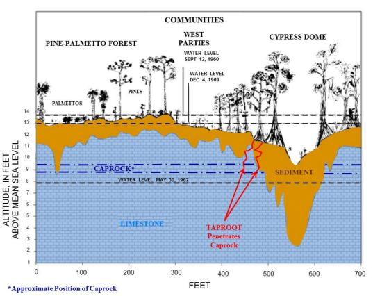
abundant presence of sloughs in the BCNP indicates that the water table intersects with the ground surface. The hydrogeology of the BCNP does not include low permeability units within the water
